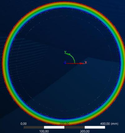
When the temperature of the flow changes by 200 °C, there is a change of the meter housing geometric dimensions, what is resulting in a discrepancy between the actual and the calculated flow rate.
