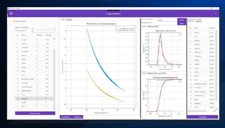
CALCULATION OF THE MOLECULAR MASS OF THE GAS OF DIFFERENT COMPOSITIONS BASED ON CALCULATION OF THE SOUND VELOCITY IN THE FLUID BY THE FLOW METER, AND ALSO THE TEMPERATURE AND PRESSURE FROM THE CORRESPONDING SENSORS.
