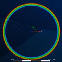
When the temperature of the flow changes by 200 °C, there is a change of the meter housing geometric dimensions, what is resulting in a discrepancy between the actual and the calculated flow rate.
